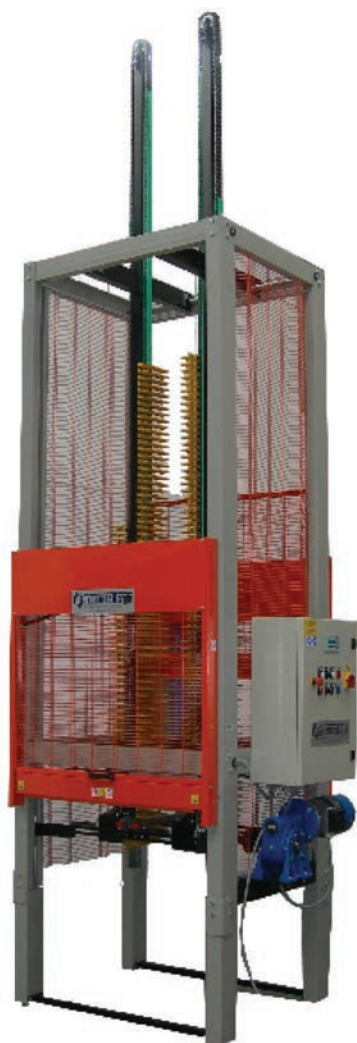
14) CMP – Compensatore verticale ad alette autoregolanti. CMP – Compensatore verticale ad alette. 14) CMP – Vertical compensator with self-adjustable tongues. CMP – Vertical slat compensator.
